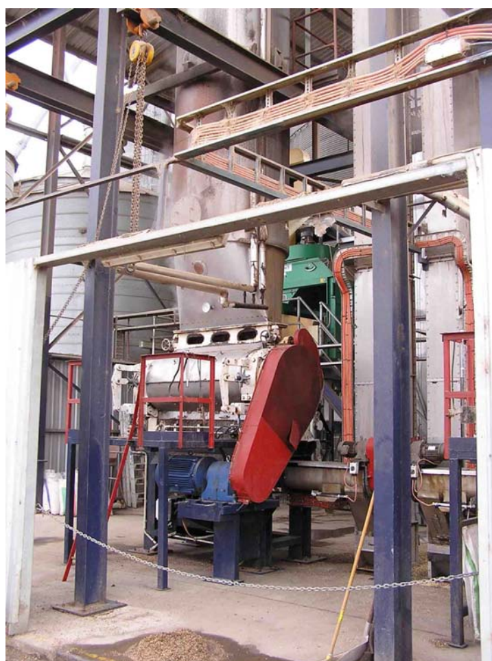
Photograph 5 – Typical grain storage and steam flaking grain processing system
