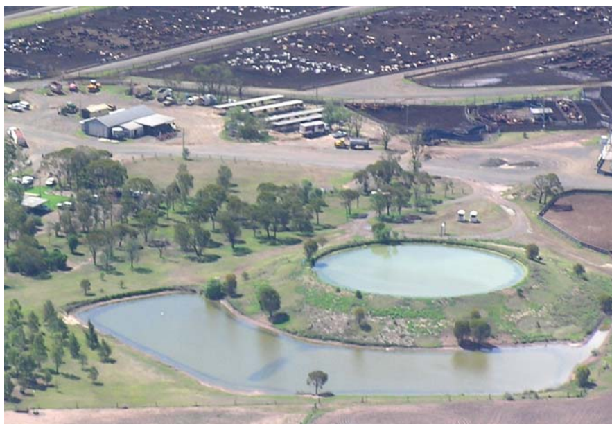
PHOTOGRAPH 5 – TURKEY’S NEST WATER STORAGE
