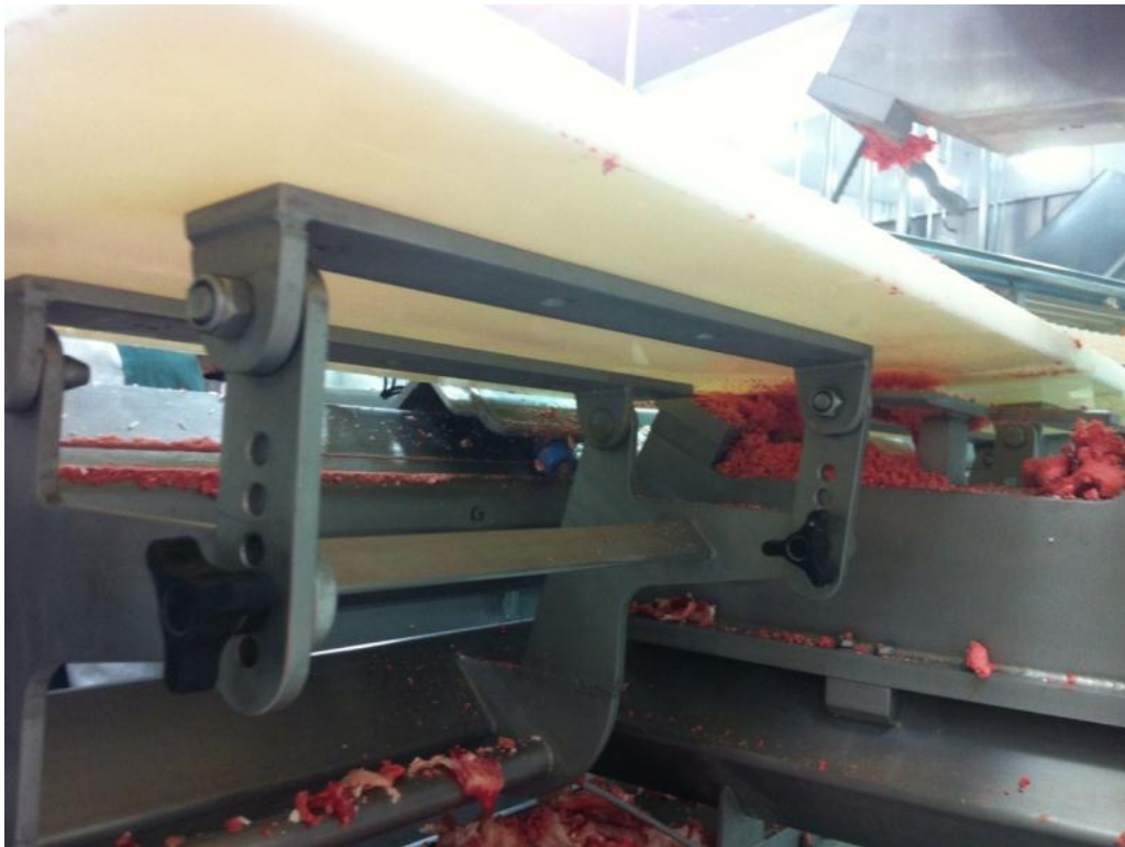
Figure 19: Adjustable table angle allows different settings for different runs of carcasses.
