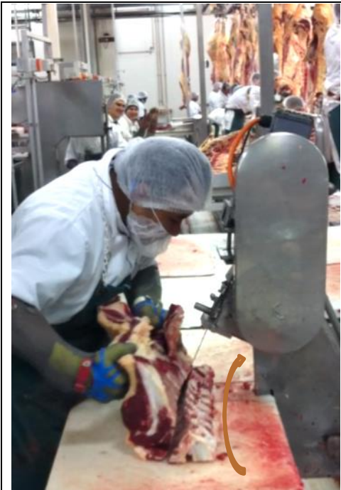
Figure 14: Cut is very close to hands and requires cut to be curved following orange arrow on picture to remove vertebrae with highest yield
