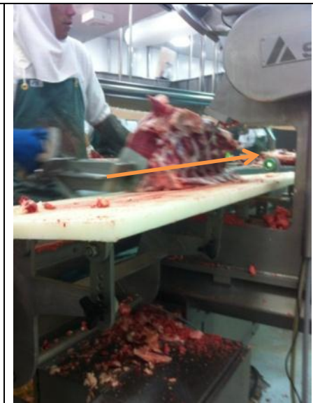
Figure 17: straight cutting line is easier for operator but could impact on yield slightly compared with generic saw although this was not evident in the data collected
