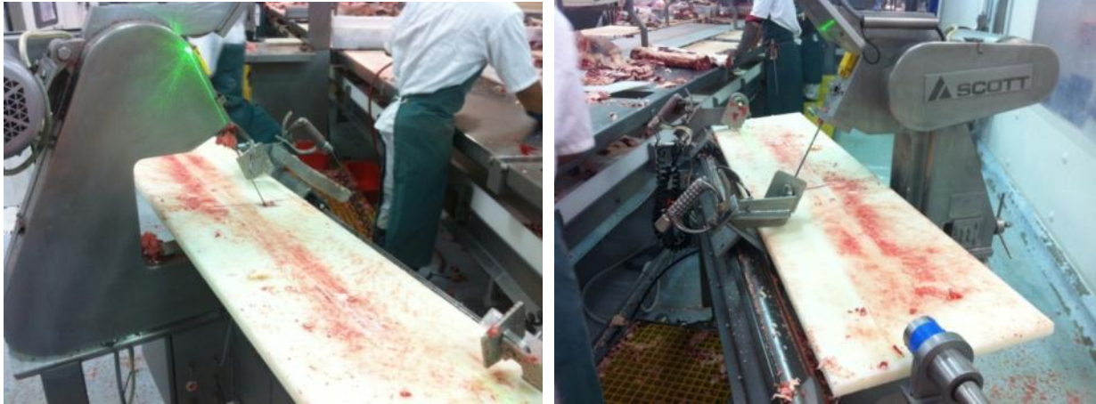
Figure 18: Integration of system into processing line will be required so operator does not have to pivot 180 degrees
