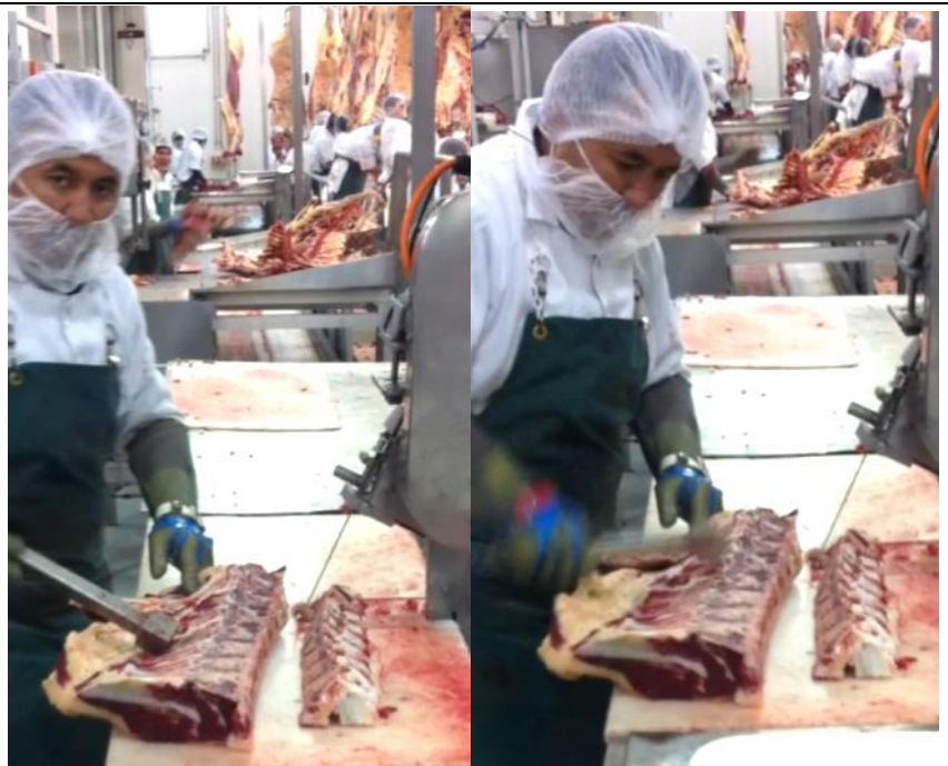
Figure 15: Steel mallet used to force the separation of ribs from vertebra where cut leaves ribs joined
