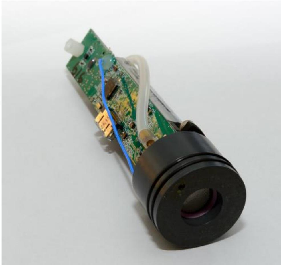
**Figure 8.** CH<sub>4</sub> and CO<sub>2</sub> IR gas-sensor device showing end-cap seals
