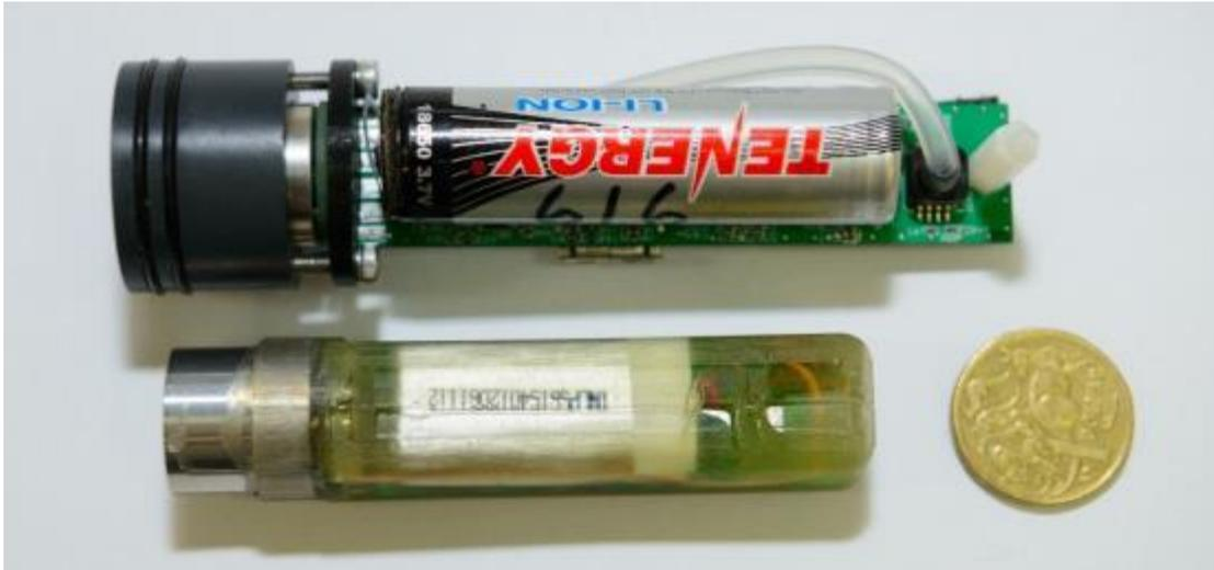
**Figure 14.** New PACP Pan wireless CH<sub>4</sub> and CO<sub>2</sub> IR gas-sensor device designed for sheep compared to the original PACP Serqet wireless CH<sub>4</sub> and CO<sub>2</sub>IR gas-sensor device
