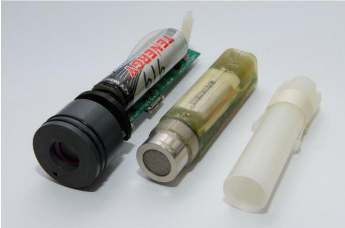
**Figure 15.** PACP wireless CH<sub>4</sub> and CO<sub>2</sub> IR gas-sensor devices and a sheep CRD
