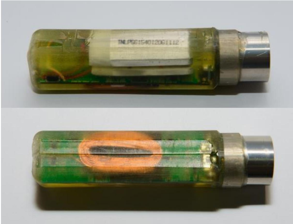
**Figure 15.** PACP Pan wireless CH<sub>4</sub> and CO<sub>2</sub> IR gas-sensor device showing batteries and the inductive charging coil
