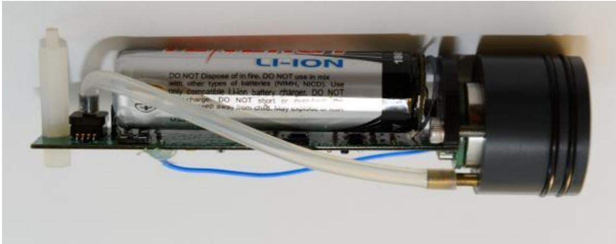
**Figure 7.** CH<sub>4</sub> and CO<sub>2</sub>IR gas-sensor device assembly
