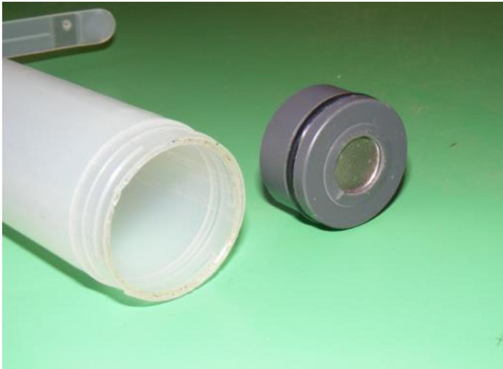
**Figure 1.** Initial CRD capsule and end-cap design
