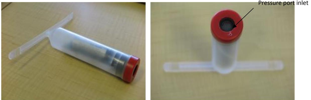
**Figure 4.** Final assembly of the current IR gas-sensing device with end-cap, PDMS membrane with supporting metal mesh is mounted onto the front of the gas sensor. Pressure port inlet is indicated.
