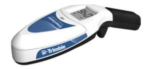
One of the critical steps is the collection of NDVI data using the Trimble Greenseeker. There is also a standard protocol for collecting the height estimate from pasture where it is required.
