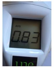
When you have finished your survey you simply take your finger off the trigger to reveal the average NDVI for the area scanned.
