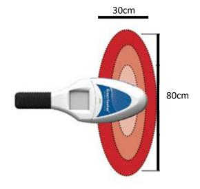
The critical point here is to ensure that the footprint of the sensor is located over the pasture and does not have your boot or part of a vehicle in it!
