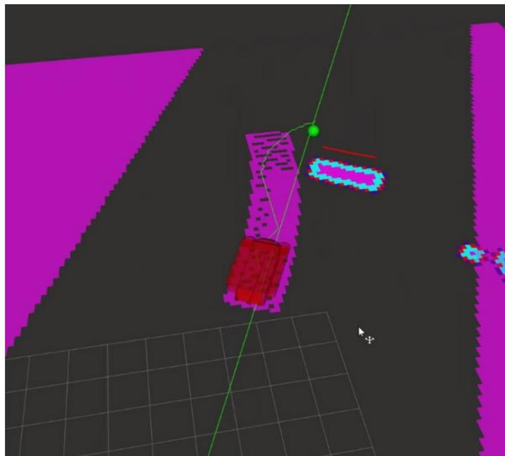
Figure 56 - Visualization of what the vehicle (red) sees as it approaches the table. As the obstacle (light blue/purple) is detected a new path is generated (green line) to go around the object. The vehicle adjusts its velocity to follow the new trajectory (purple path).
