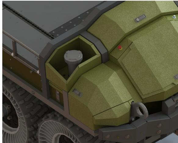
Figure 23. Phase II front fuel fill, box lid hidden for clarity.
