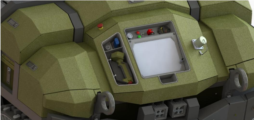
Figure 15. Phase II RC storage location and battery charger, cover hidden for clarity
