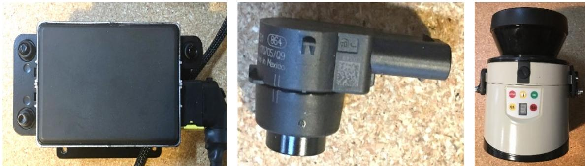
Figure 37 – From left to right: RADAR, Sonar, LiDAR
