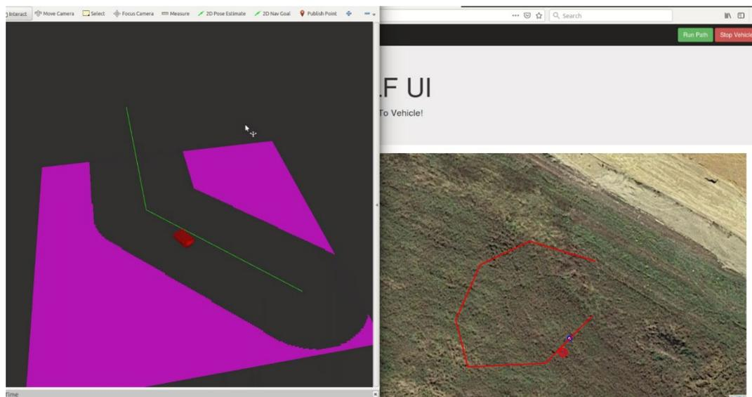
Figure 54 - Waypoint navigation. The image on the left is for visualization purposes and displays the vehicle (red) traversing the path (green) and the outer edges of the road (purple). The image on the right is a part of the GUI displaying the total path (red line) with the vehicle (red circle).
