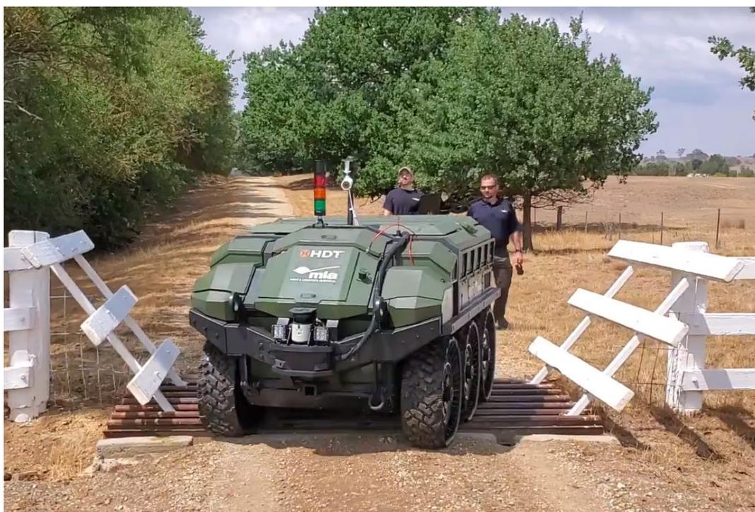
Figure 62 - System navigating through gate over cattle grid
