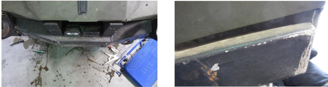
Figure 19 – (left) Phase I front bumper (right) Phase I front bumper wear.
