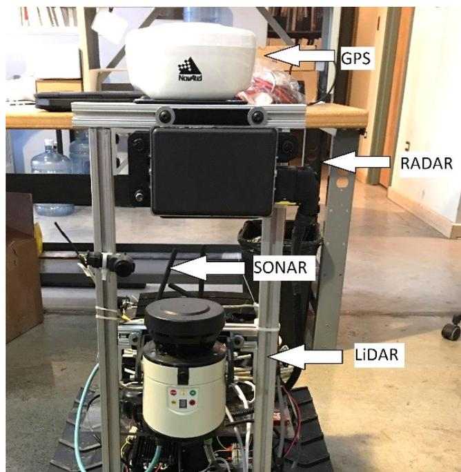
Figure 38 - Test vehicle fitted with the sensors described above (front view)
