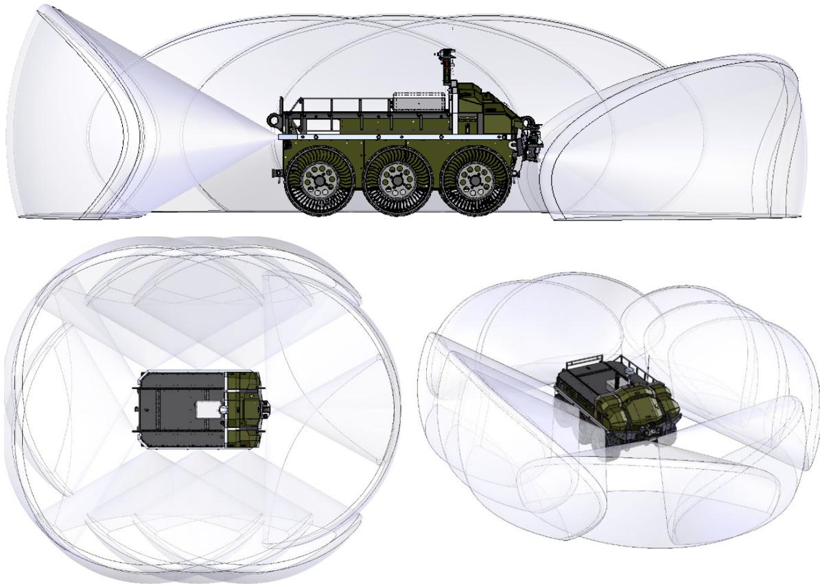
Figure 41 - Top view of Wolf showing coverage area of 10 ultrasonic sensors
