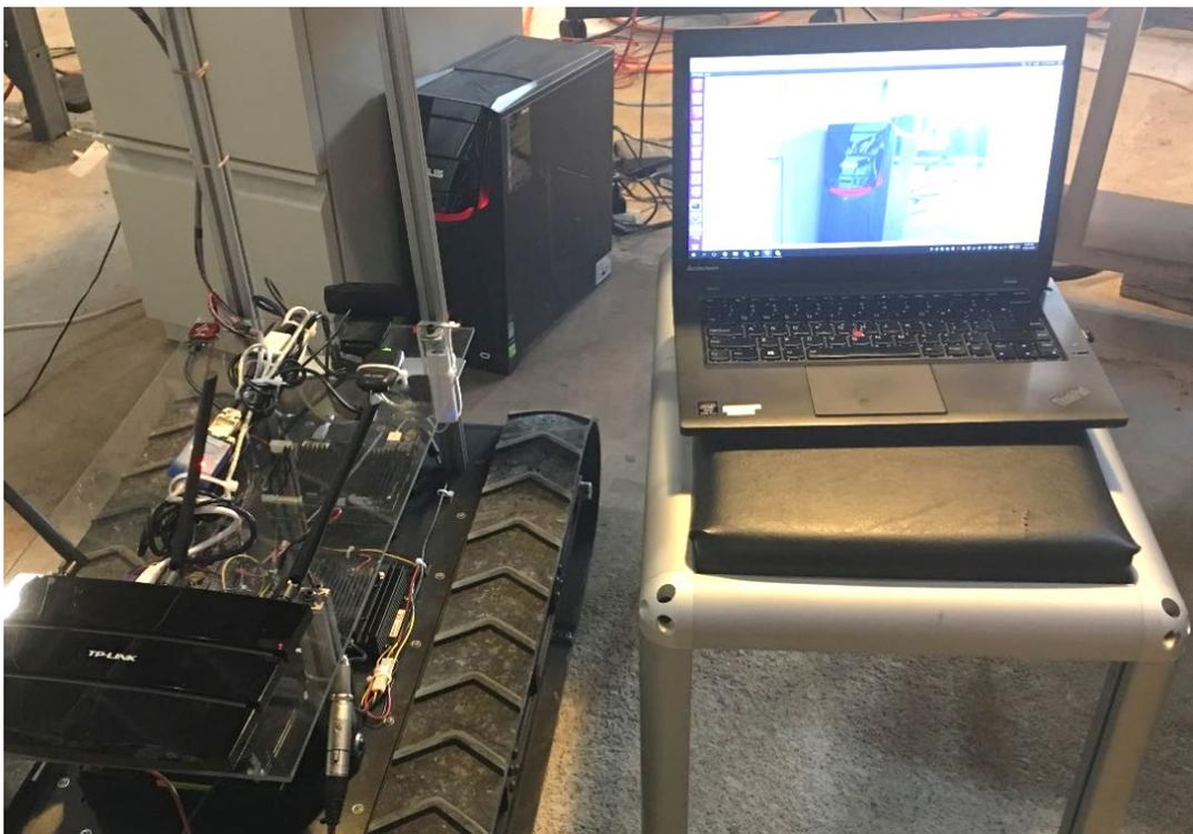
Figure 46 – Picture demonstrating a view of the test vehicle streaming data onto a laptop.
