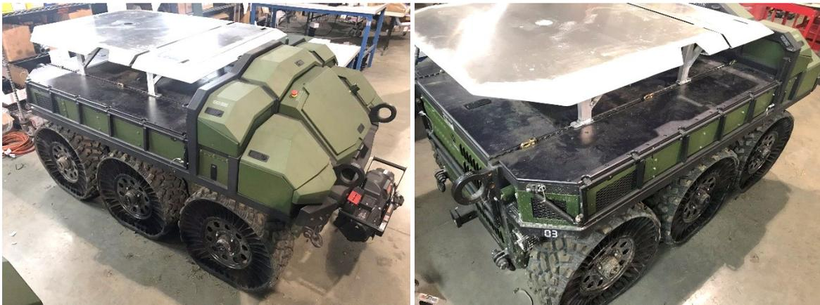
Figure 35 - Flight Deck test fit onto WOLF
