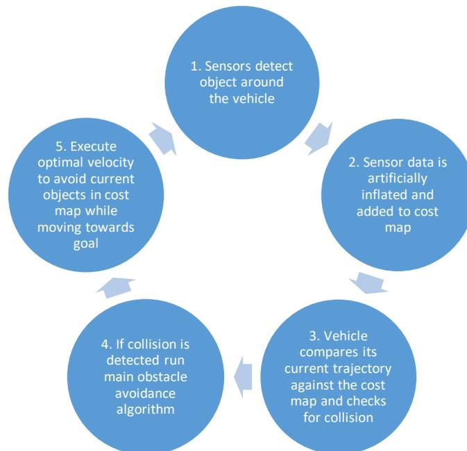
Figure 47 - Flow Chart providing basic idea of how obstacles are detected and avoided
