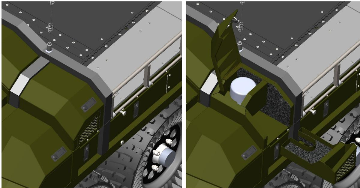
Figure 10 – (left) Phase II air intake, closed (right) Phase II air intake, open, tray removed (baffling and foam shown)
