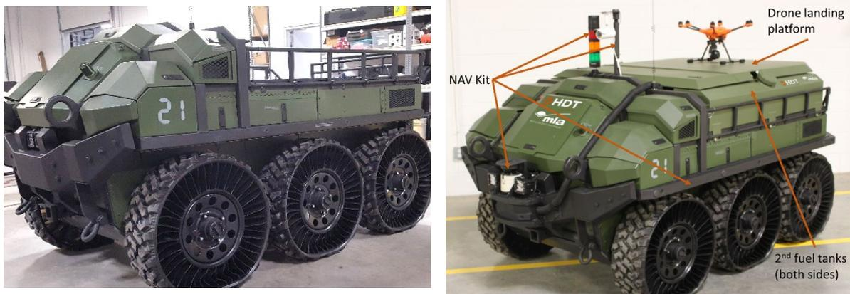
Figure 53 – Pictures of the (left) baseline Hunter WOLF vehicle, and (right) Drover WOLF integrated with the NAV Kit, secondary fuel tanks, and the drone platform.
