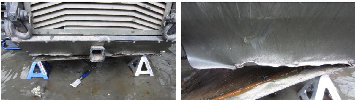
Figure 21 – (left) Rear skid plate damage (right) Front skid plate damage
