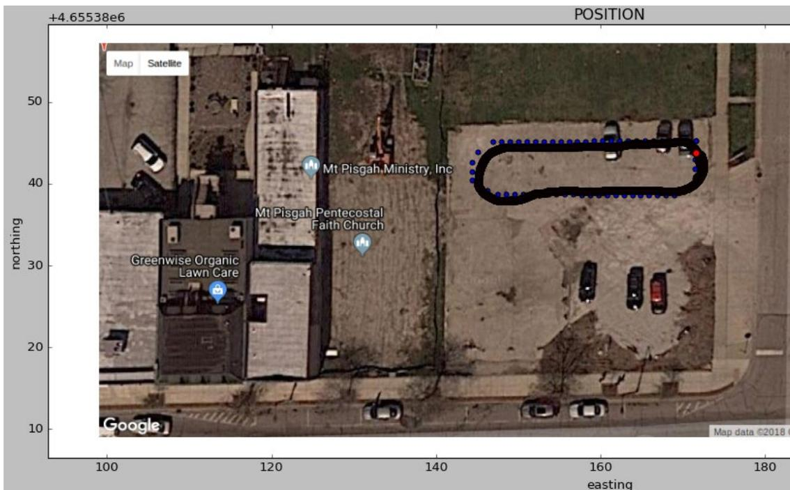
Figure 36 – Result of path tracking algorithm. Desired path consists of the blue dotted path, actual path traversed in black
