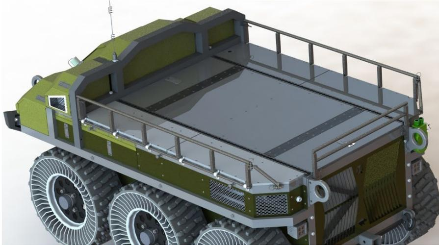
*Figure 22. Phase II Side Rails in the raised position.*
