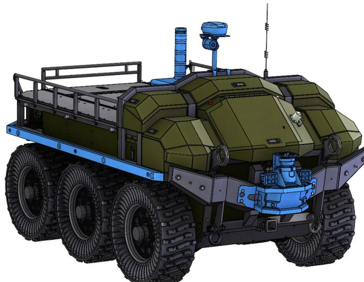
Figure 40 - Final Design of WOLF autonomy package highlighting the autonomy components (in blue)
