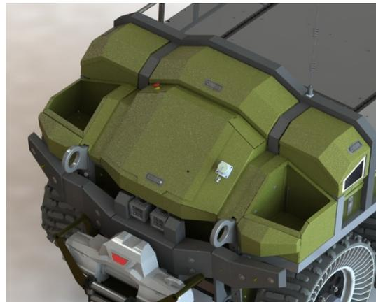
Figure 18 – (left) Phase I BMS location, lid hidden for clarity. (right) Phase II front fender storage boxes, lids hidden for clarity
