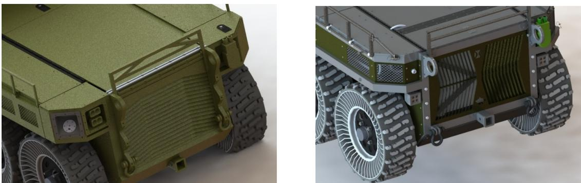
Figure 14 – (left) Phase I louvers (right) Phase II Louvers
