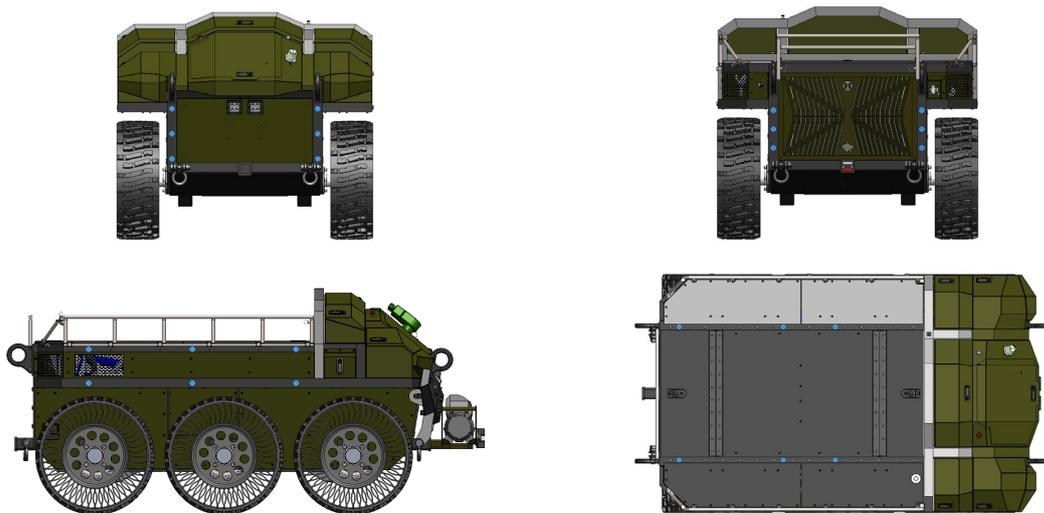
Figure 8 – (top-left) Phase II front: 6x M10 Mount Points (bumper hidden to show). (top-right) Phase II Rear: 6x M10 Mount Points. (bottom-left) Phase II sides: 6x M10 Mounts Points on Each side. (bottom-right) Phase II deck: 6x M12 Mount Points (aircraft tracks hidden to show)
