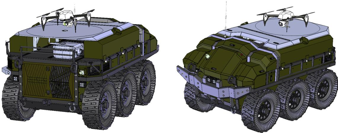
Figure 33 – (left) Wolf with drone landing pad. Shown with auxiliary fuel tanks. Rear view. (right) Wolf with drone landing pad. Shown with auxiliary fuel tanks. Front view
