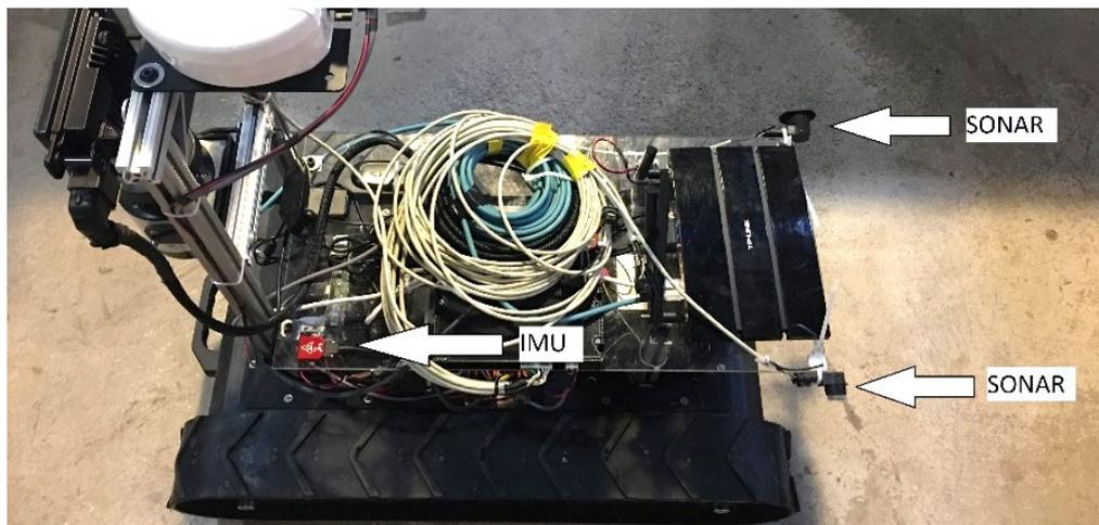
Figure 39 - Test vehicle showing the IMU and two additional sonars for collision detection in the back of the vehicle
