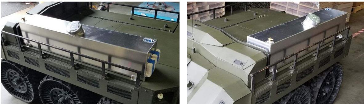
Figure 32 – Pictures of the base vehicle with 1 auxiliary tank installed.
