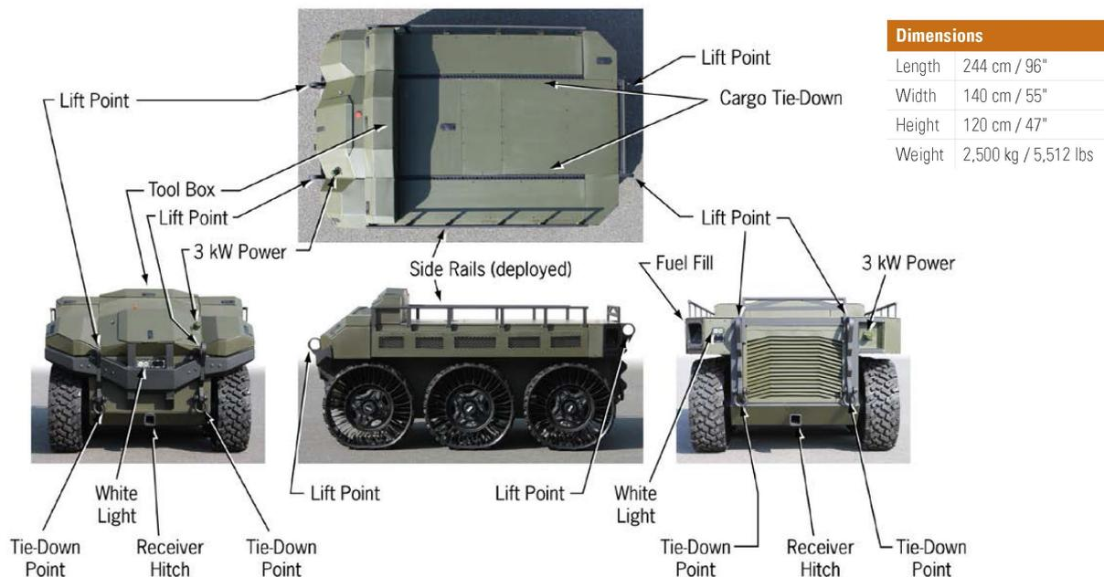
Figure 67: HDT's Hunter WOLF unmanned vehicle is about the same size as a large quad bike, but far more powerful and stable.
