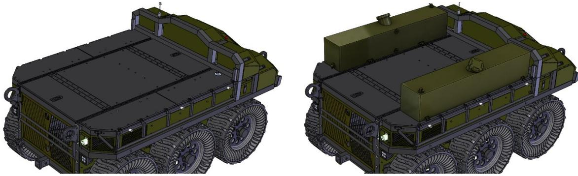
Figure 31 – (left) Base vehicle; 456 km range (flat road). (right) Base vehicle with additional fuel tanks; 1369 km range (flat road).
