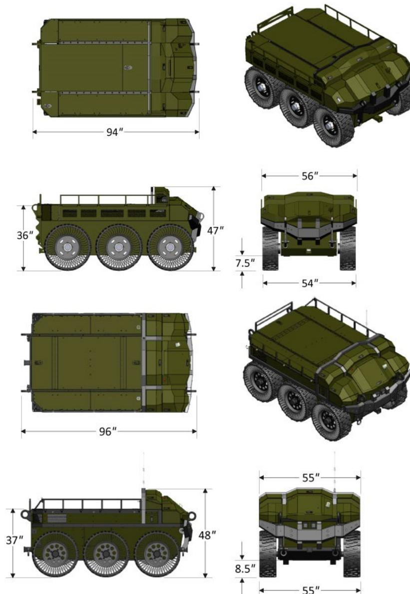
Figure 5. (top) Phase I and (bottom) Phase II Hunter WOLF vehicles dimensions
