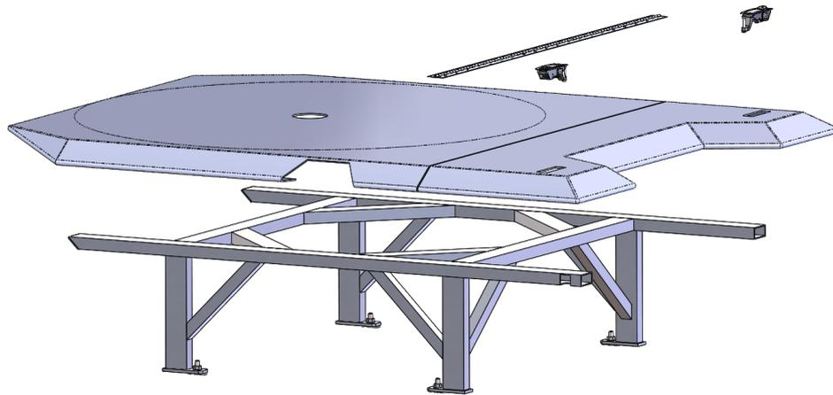
Figure 34 - The main parts of the landing pad
