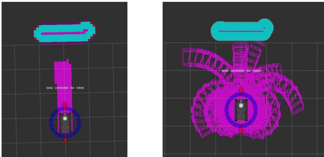
Figure 50 - Vehicle driving towards an obstacle(light blue). Image on the left shows the desired trajectory (purple) before a collision is detected. Image on the right shows the discretised trajectories (purple) considered after a collision is detected
