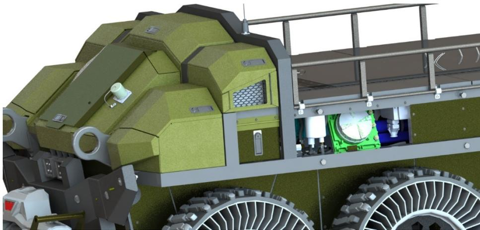
Figure 17. Phase II fuse box (green), access panel door hidden for clarity
