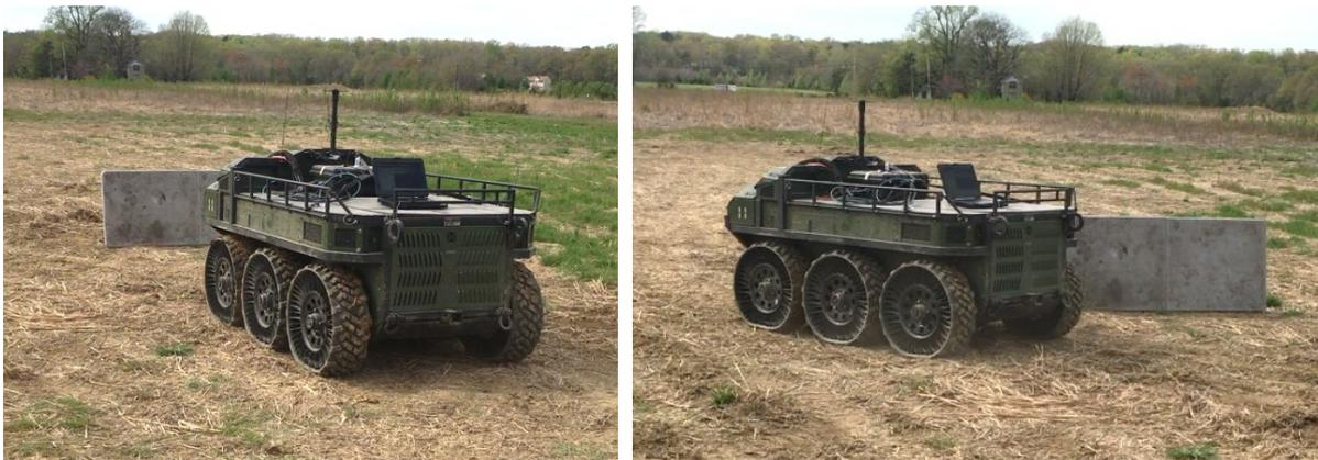
Figure 55 - WOLF Approaching a table laying on its side on the left. Navigating around it on the right.
