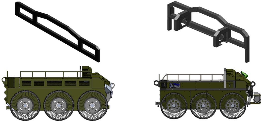
Figure 6 – (left) Phase I Rollbar. (right) Phase II Rollbar
