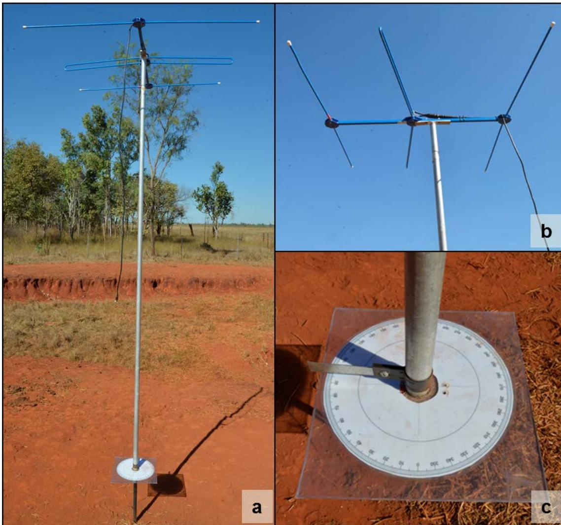
Figure 41. Triangulation towers consisting of an 18 mm diameter x 50 cm length metal rod driven on the ground with a hammer. (a) Shows the complete tower; (b) 3 element folding Yagi antenna (Sirtrack Ltd) aligned to the needle and fixed to the pipe by an aluminium handle that slide into the aluminium pipe forming the tower; and (c) Plastic protractor calibrated true north and showing the needle and bracket.
