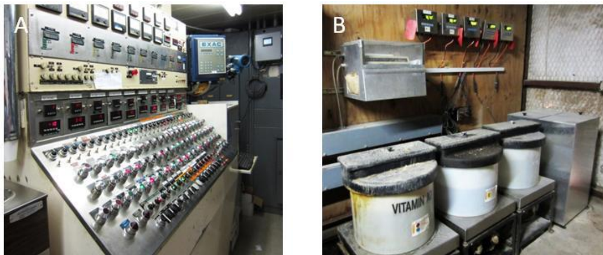
Figure 7.8. Components of the ration mixing system installed at the Kirkland Feedyard, Texas. A. . Feed mixer controller system. B. Bins of micro-ingredients supplying the Comco micro-feeder system.
