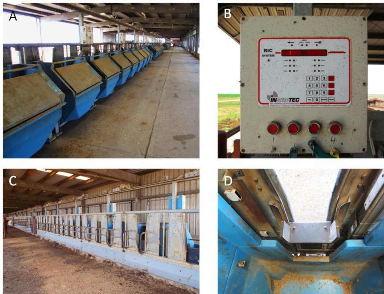
Figure 7.14. Insentec feed system installed in the research pens at the MARC, Clay Centre, Nebraska. A. External face of the feed bins. B. Controllers and data logger. C. Pen-side view of the feed bins. D. Internal view of a feed bin reveals the weighing system and ear tag readers.
