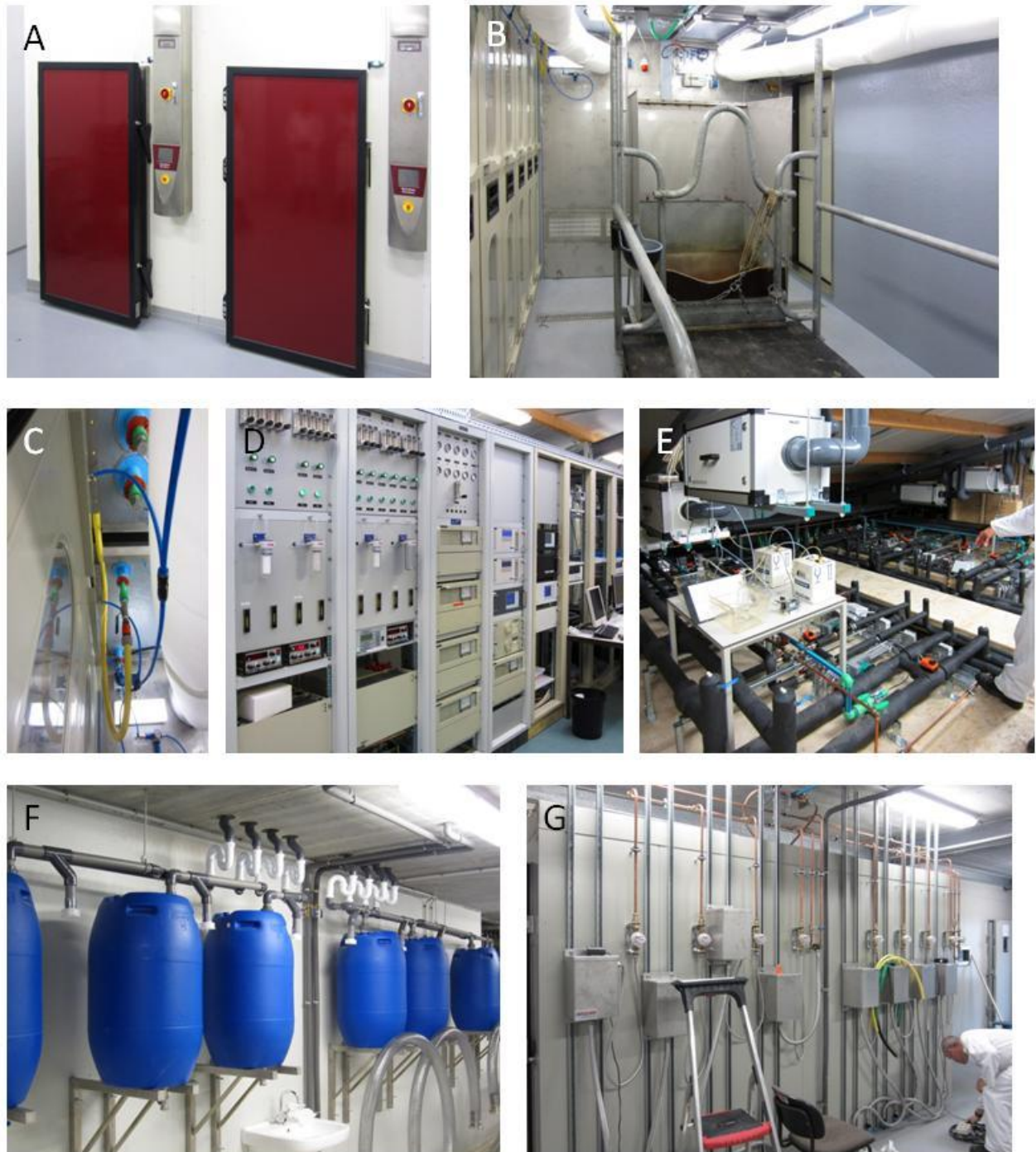
Figure 7.16. Recently installed and commissioned metabolic chambers at the Wageningen University, Department of Animal Sciences. A. External doors into the individual chambers. B. Internal view of an individual chamber. C. Compressed air lines supplying the internal door sealant system. D. Automated on-line gas chromatographs and controllers units supporting the chamber operation. E. Supporting pumps, lines and valves above each individual chamber. F. Urine and faeces collection containers below the chambers. G. In-flow and out-flow gas and air lines leading to and from the individual chambers.
