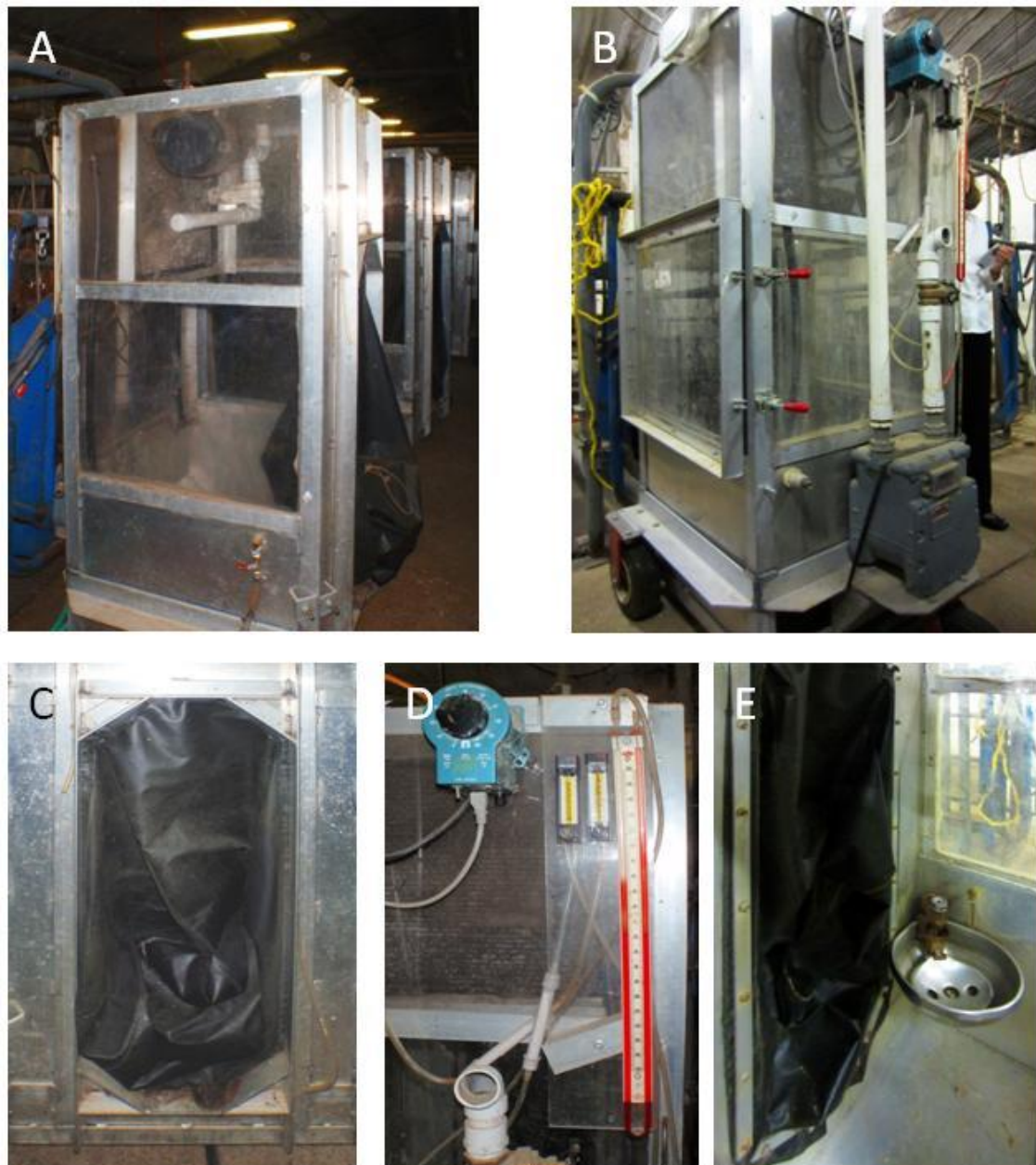
Figure 7.12. Indirect calorimeters housed in the climate chamber at the MARC, Clay Centre, Nebraska. A and B. Indirect calorimeters. C. Head sleeve. D. Temperature and %RH measurement. E. Low flow water feeder installed in the calorimeter.
