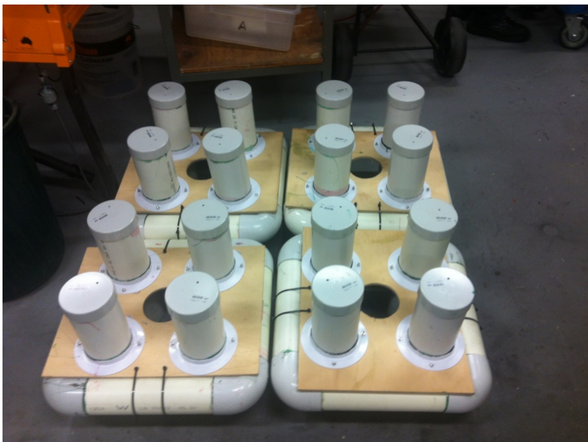
Figure 2 Sampling rigs deployed on the Kerwee pond for sampling of biogas for the manual estimation of rate of methane emission.
