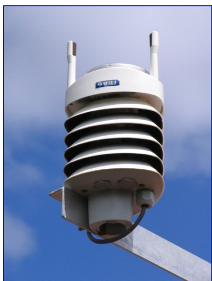
Figure 7 The Vaisala WXT520 weather transmitter.
