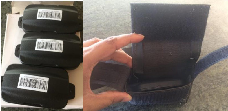
Fig.1 : LoRaWAN GPS Sensor Module + Cattle Collar
