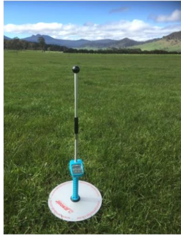
Fig. 4. Electronic pasture plate meter used to measure kgDM/ha at “Elverton”
