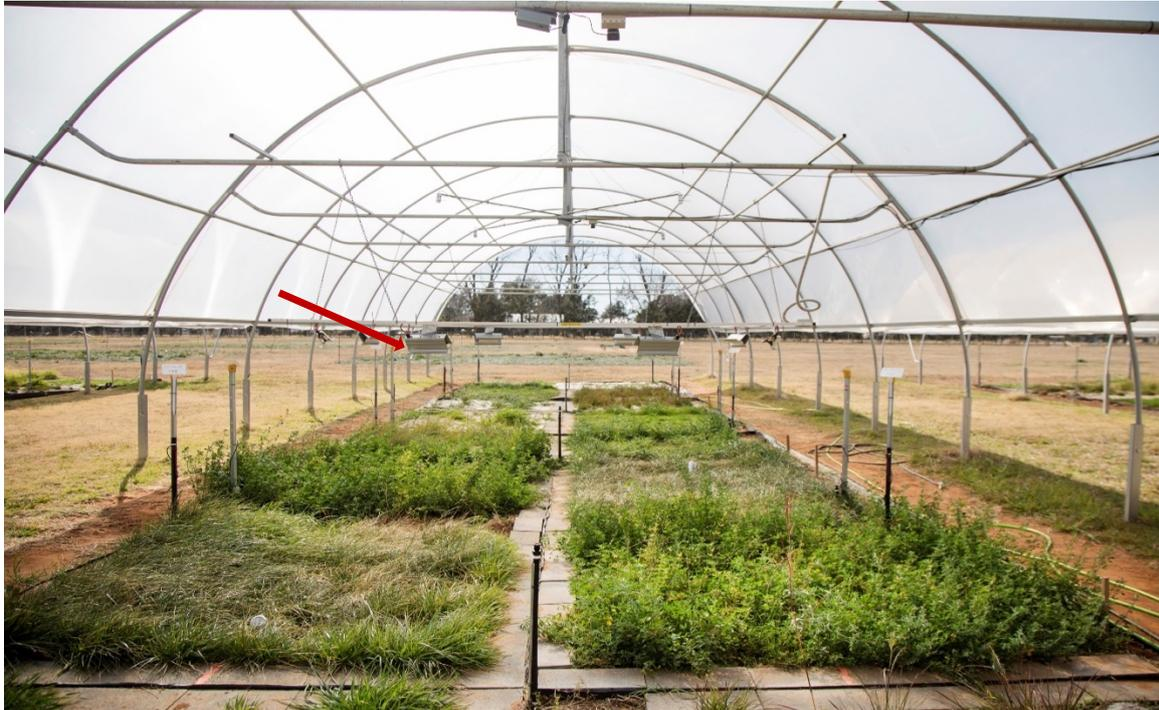
**Fig 1.** Interior of a shelter at the PACE facility showing different pasture subplots. The IR heating array (with ceramic lamps - red arrow) for the + 3 °C treatment is visible in the centre of the image.
