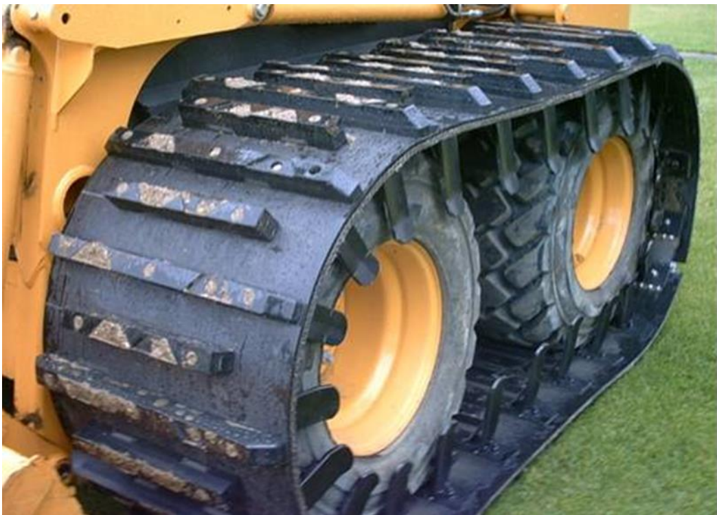
Figure 8 – commercial skid steer track kit from Right Track showing belt, external grousers, and internal wheel guides.
