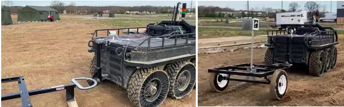
Figure 48 – (Left) Once in position, the hitch is engaged in order to pick up the trailer. (Right) with the trailer hitched, the vehicle drives away to its next goal.
