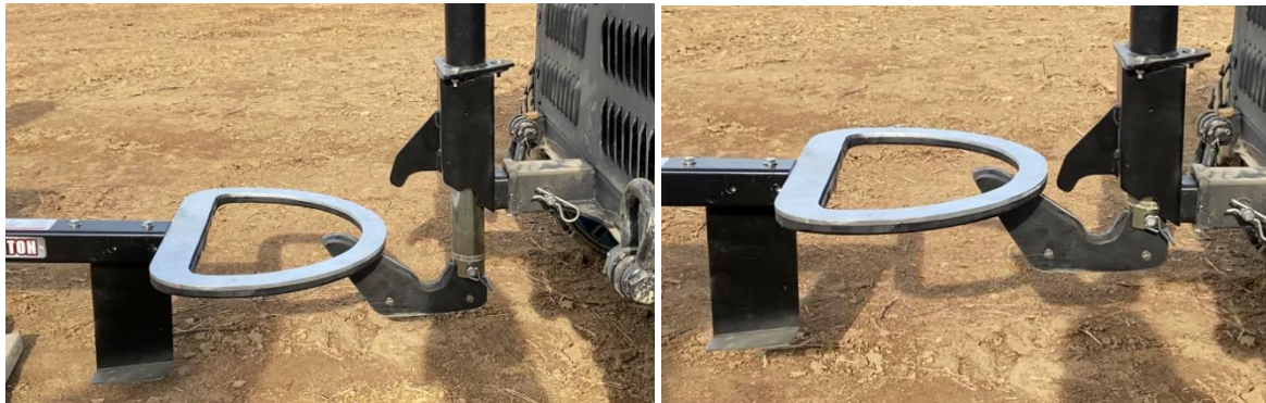
Figure 49 – (Left) while being hitched it may occur that the trailer does not slide into the groove on the hitch. (Right) The trailer is left unsecured – and is likely to fall as the vehicle begins to move – as a result of it not sliding into the groove.
