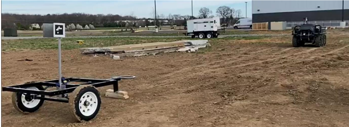
Figure 46 – Initial demo state. The WOLF has arrived at a location near the trailer, and is now ready to begin the hitching process.
