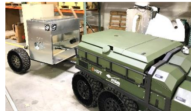
Figure 1 – (top) Picture of Protector (the precursor device), (2 nd from top) Hunter WOLF v1, (3 rd from top) Drover WOLF (v2); vehicle which integrates the autonomous navigation kit, (bottom) Drover WOLF integrated with the dry-supplements distribution system.
