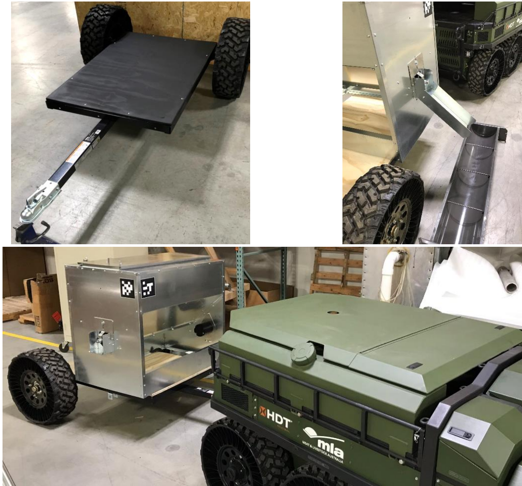
Figure 29 – (top left) Picture of the modified COTS trailer. (top right) Picture of the Drover WOLF integrated with the trailer, Stall feeder and hitched to the WOLF. (bottom) Picture of the integrated system.
