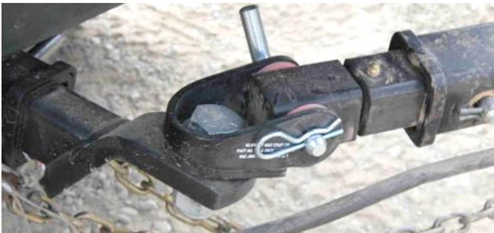
Figure 34 - Hitch with 3 degrees of freedom
