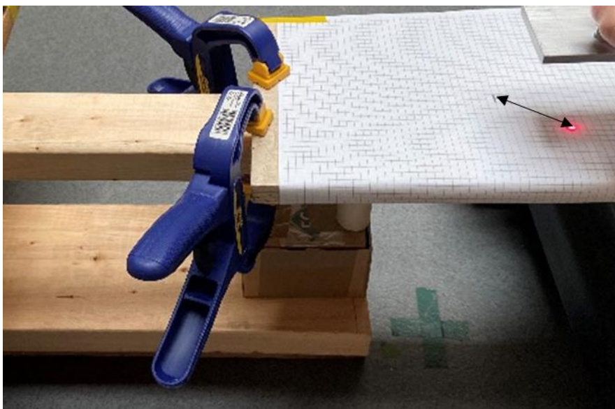
Figure 44 – Accuracy was measured using a laser pointed at a gridded sheet of paper after each test run.
