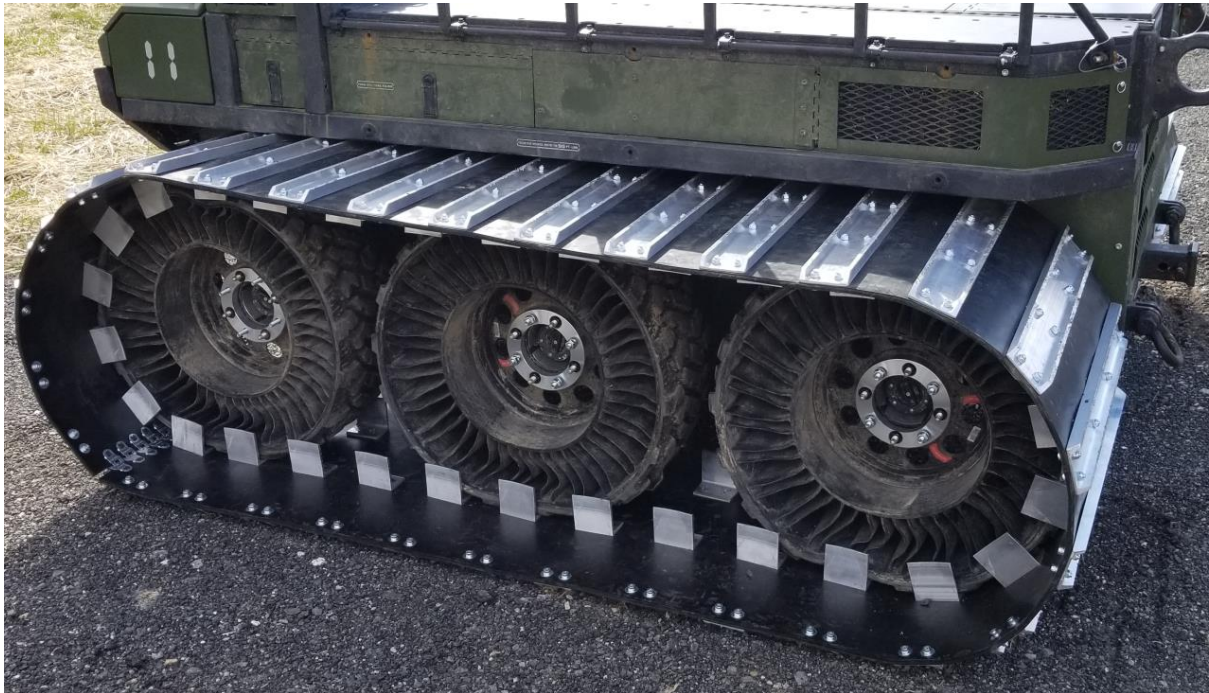
Figure 14 - LGP track installed on test vehicle
