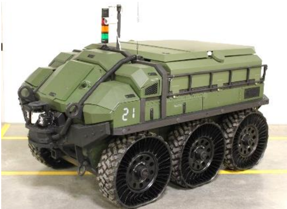
Figure 5 – HDT Drover WOLF (i.e. Hunter WOLF with AUV deck, waypoint navigation (NAV) kit, and additional fuel tanks.)
