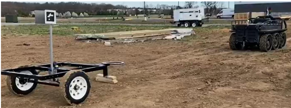
Figure 47 - (Top) Vehicle begins to look for fiducials by approaching the trailer GPS location with the rear facing camera in front. (Bottom) The vehicle spots a fiducial and stops in order to record its pose. With this information the vehicle can now be sure of where the trailer is.
