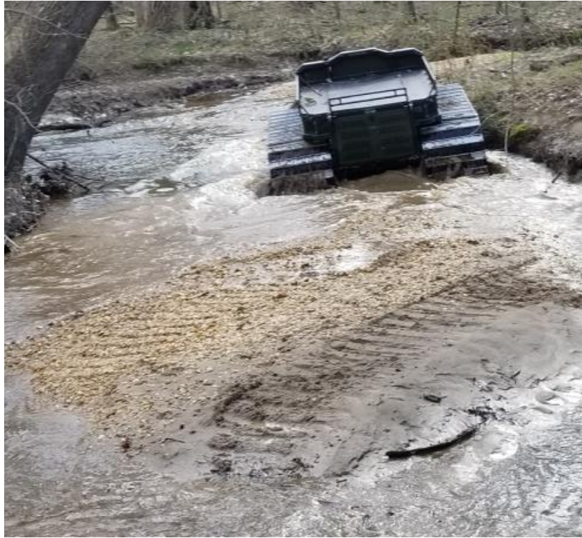
Figure 16 - Test vehicle in a stream, showing minimal tracks on gravel and silt bed
