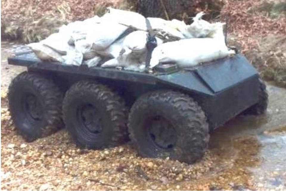
Figure 3 – Picture of MadDog, a battery only wheeled initial prototype
