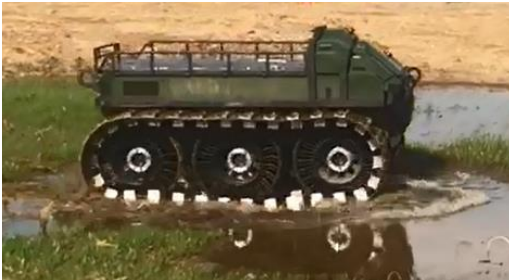
Figure 7 – Picture of the WOLF using the Low-ground pressure kit.
