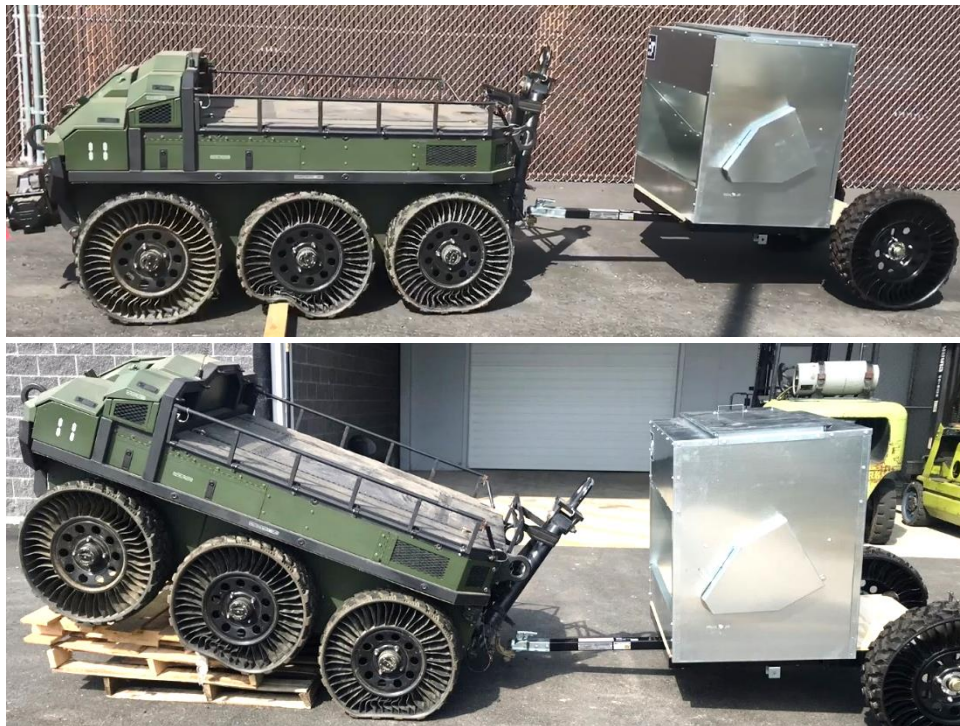
Figure 30 – Pictures of early testing that was performed to confirm strength and stability of trailer as well as the range of motion of the hitch.
