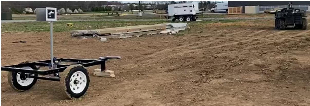
Figure 46 – Initial demo state. The WOLF has arrived at a location near the trailer, and is now ready to begin the hitching process.
