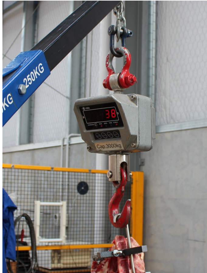
Fig. 5: A load cell allowed control over the mechanical load applied to the spine during the cut
