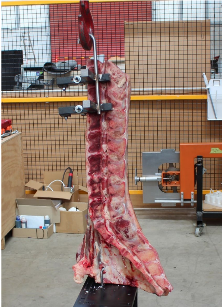
Fig. 4: Clamping setup for the rump and loin sections used in the workshop trials
