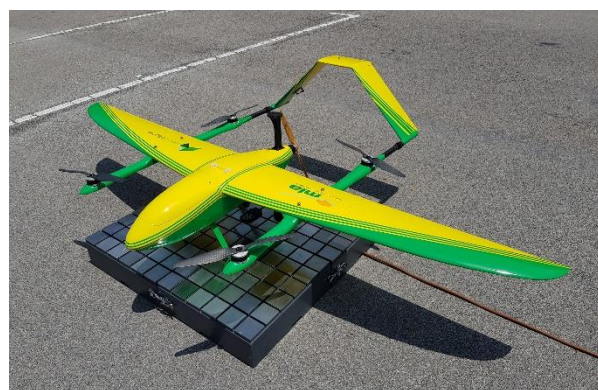
Fig. 10: Ground test for charging pad
