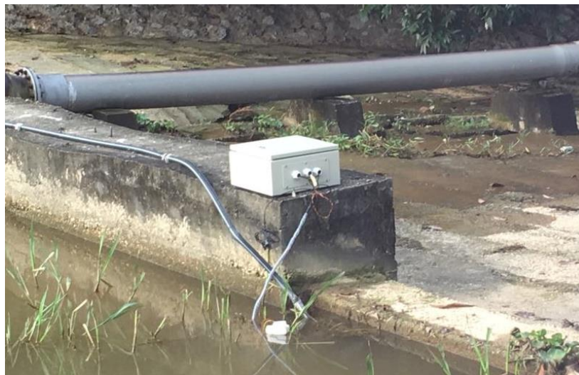
Fig. 54: Enclosure box with the sensors immersed
