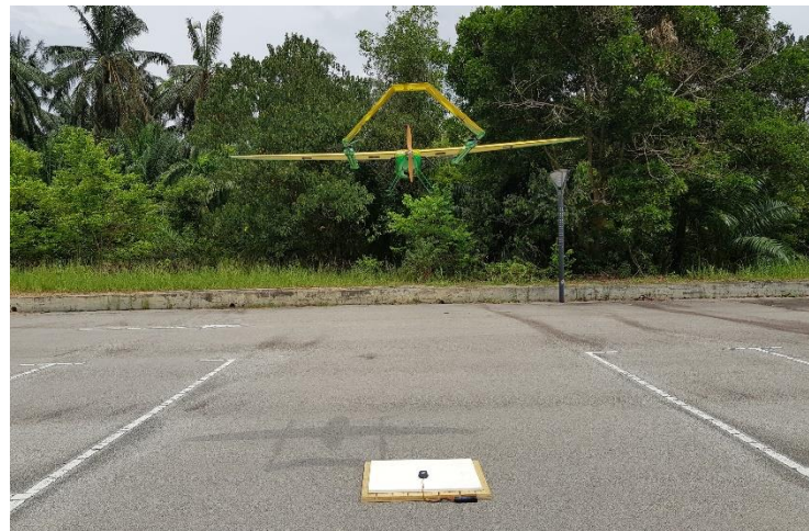
Fig. 6: The VTOL drone trying to lock its position and land above the beacon
