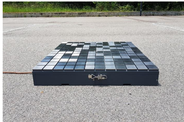
Fig. 9: Assembly of four individual charging pads
