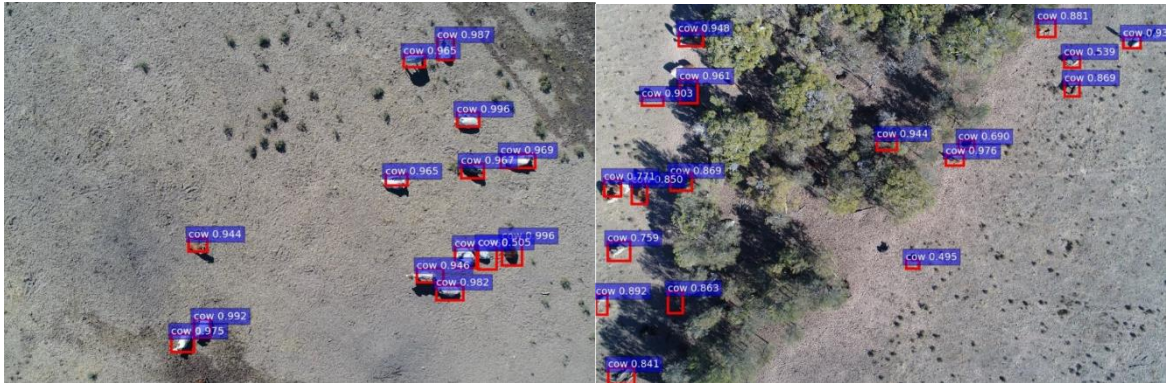
Fig. 37: Cow detection from drone aerial view at 30m altitude, less density (left); high density (right)
