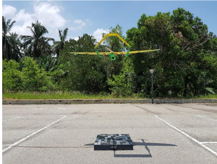
Fig. 11: VTOL drone trying to land on top of the charging pad
