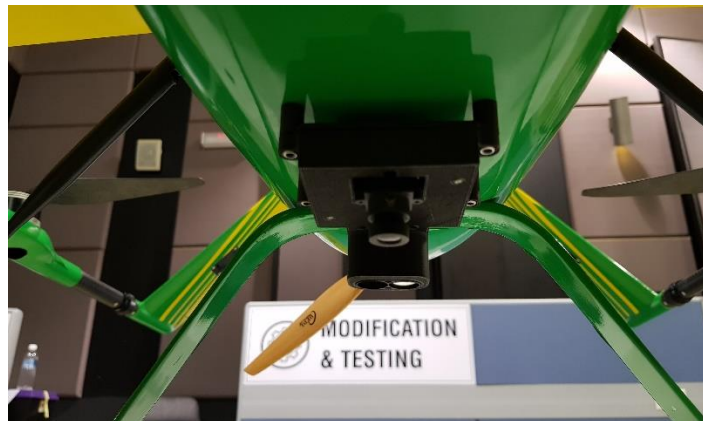
Fig. 5: Precision landing system mounted on the VTOL drone
