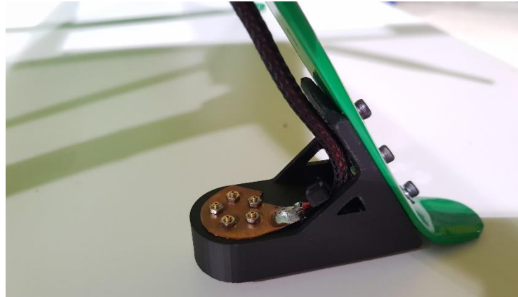
Fig. 8: Close up view of contact charging kit
