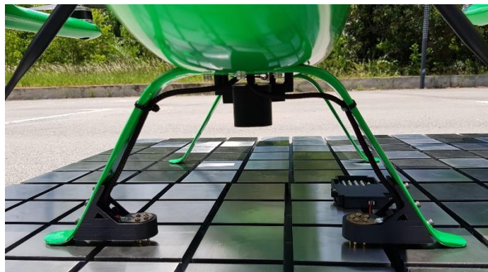
Fig. 36: Camera position as compared to the beacon
