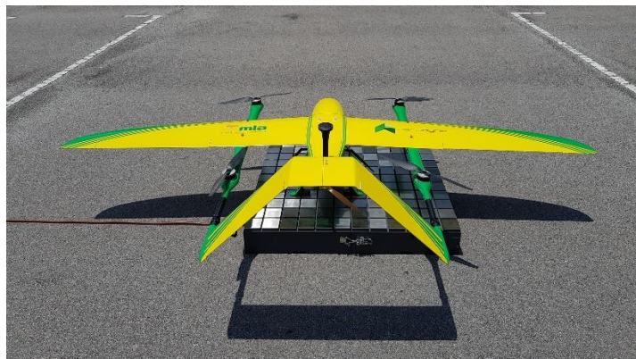
Fig. 35: VTOL drone position on the charging pad
