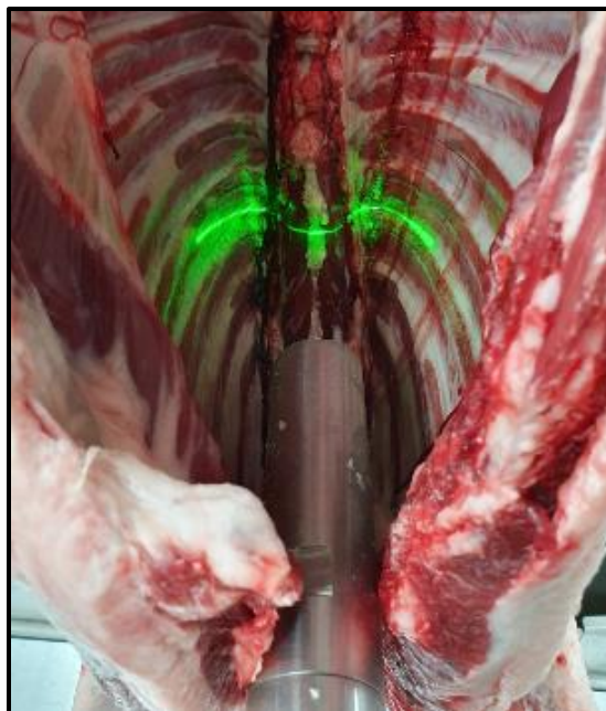
Fig. 18: Manual measuring station targeting FQ ribs with laser projection.
