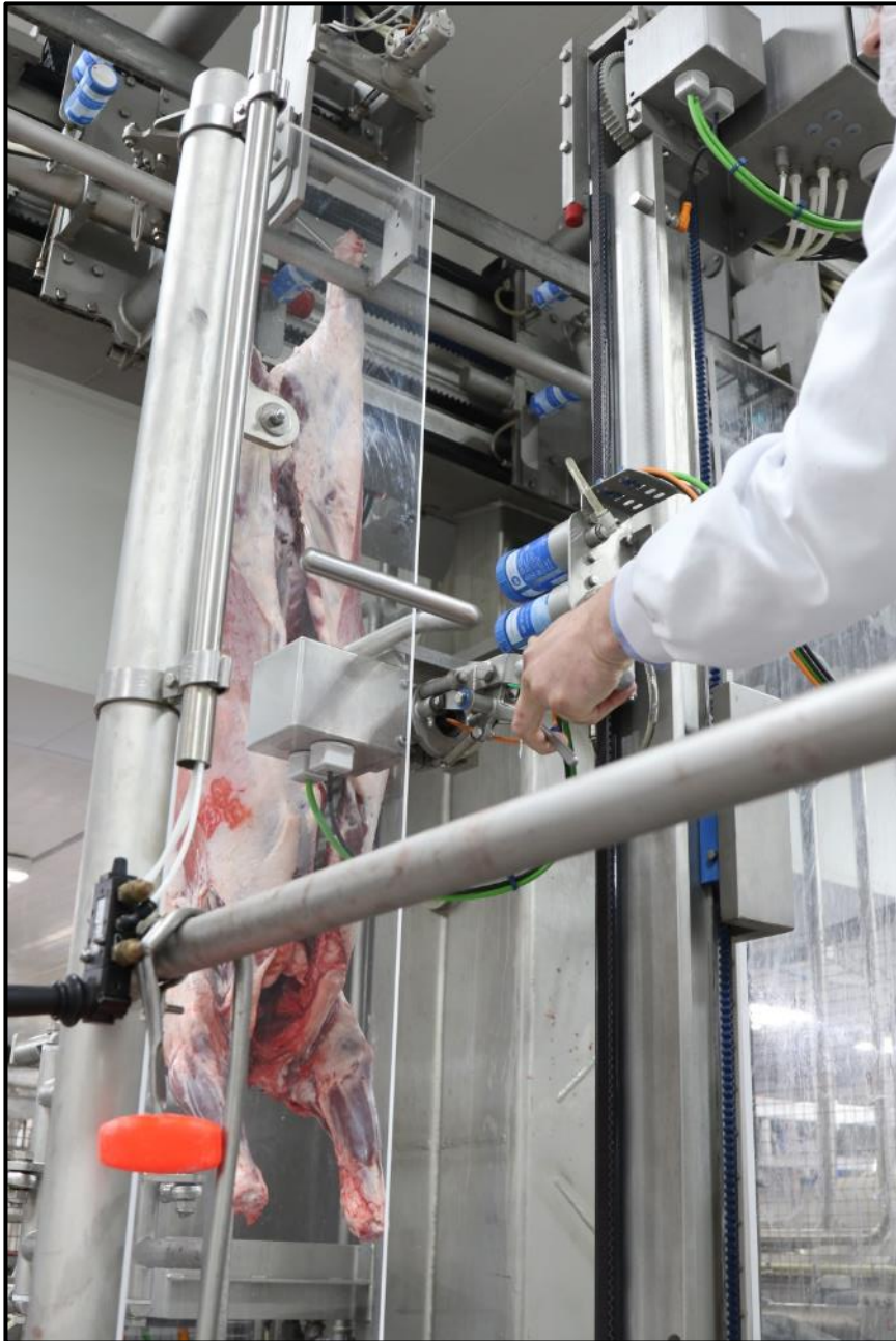
Fig. 35: The operator moving the laser to different cut positions
