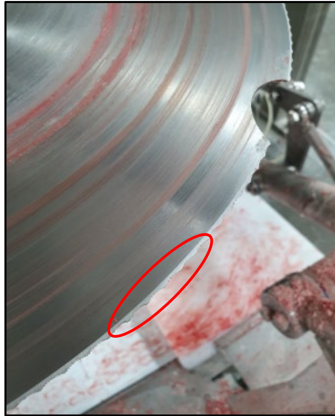
Fig. 24: Blade fracture on BE Blade, with section of dulled teeth prior indicating likely cause of fracture was contact with metal object
