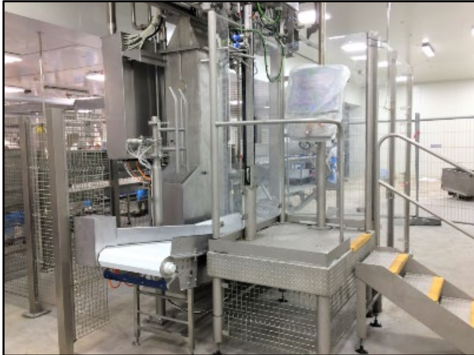
Fig. 19: Fencing installation on the 21/9/2018 with the infeed and outfeed product rails still missing.
