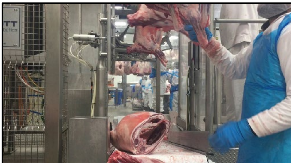
Fig. 37: Cut product (Saddles, FQ's) being fed out of machine on conveyors
