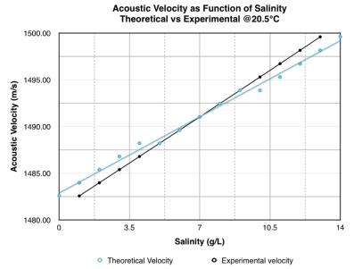
Applying our algorithm on the experimental acoustic velocities yields a close approximation of actual salinity (see below graph). It should be noted that for salinities less than 2g/L the readings become increasingly less accurate. Due to the intended use of this sensor this is acceptable as expanded on in the discussion below.
