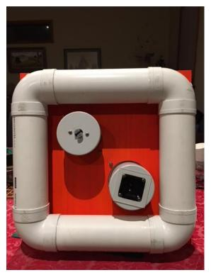
BGA Top: IP67 rate housing with LoRa antenna – includes the BGA sensor. The second shorter cylinder houses the Turbidity sensor.
