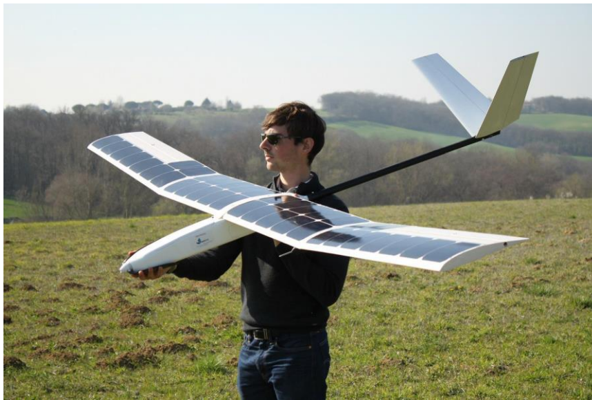
Figure 20: The Sunbird™ Solar Powered drone with 8 h endurance
