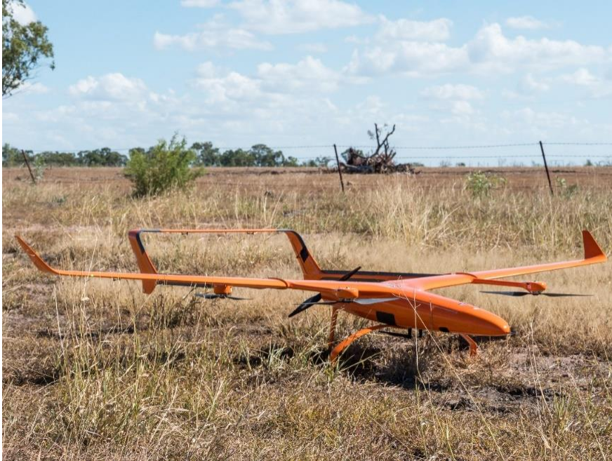
Figure 19: The Volanti™ with its 3.2 m wingspan and 2 h flight endurance
