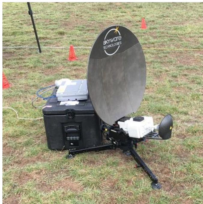
Figure 15: Atom 65a Satellite Transmitter used at Carwoola
