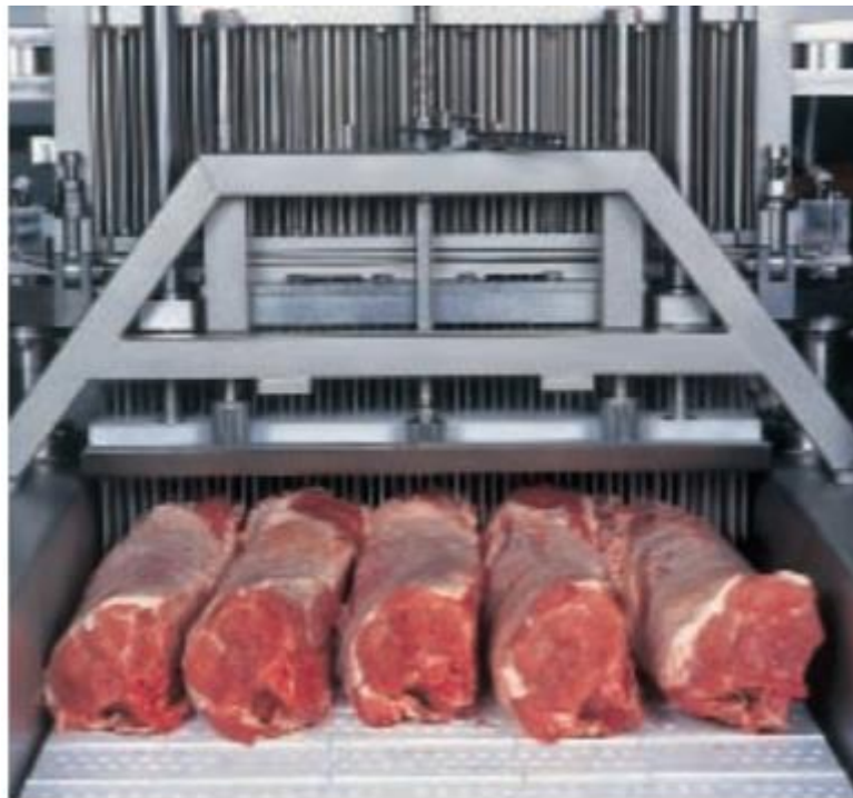
Figure 7: Meat injectors with adaptation for gas injection
