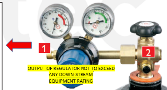
Example: Flavourless Smoke Cylinder Pressure filled to minimum 1015 psi ~ 70 Bar.
