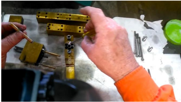
*Hide-stamper's pistons being replaced + a Veal Bleed Chain Lifter receiving maintenance, performed by an older worker, who owns the knowledge around these critical equipment processes.
