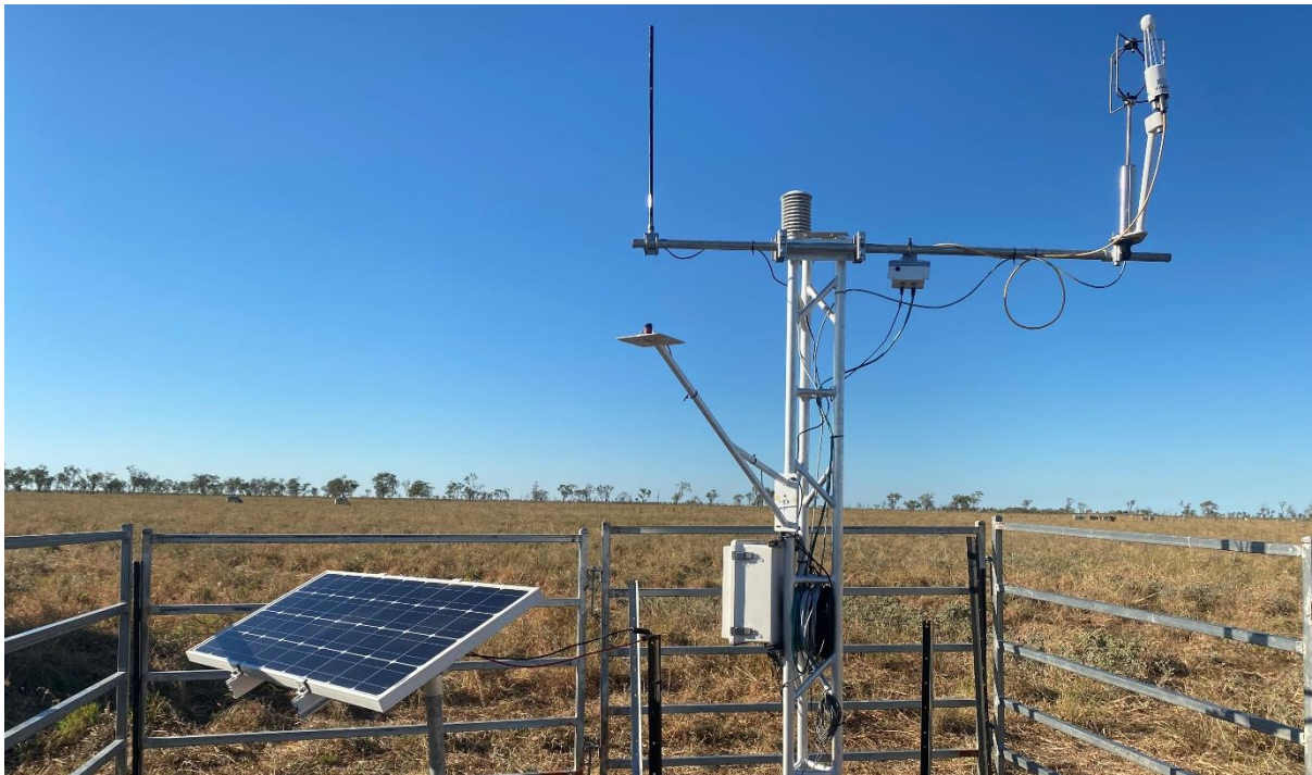
Figure 7 Eddy co-variant flux tower at the Gregory Downs soil carbon project
