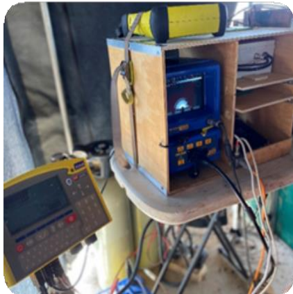
Figure 2 Martins Ewe Scan, Preg Scanning unit equipped to record Preg Status, litter size and foetal aging using eID.
