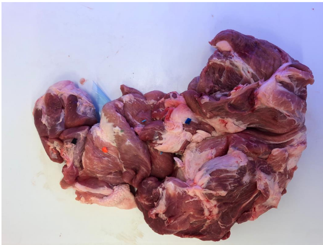
Figure 6: Test piece of beef including transparent blue poly, blue poly foreign objects, ear-plug, and ear-plug string.
