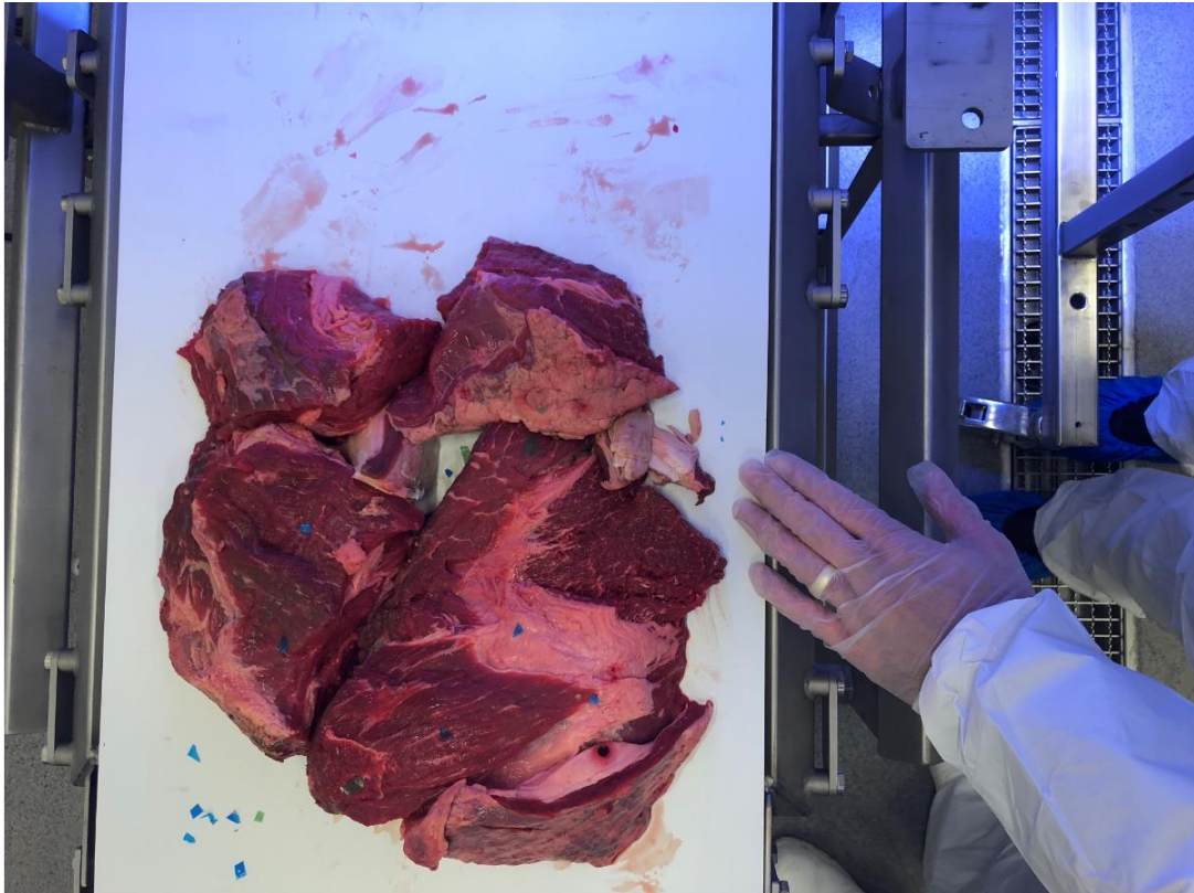
Figure 5: Test piece of beef including blue poly and transparent green poly foreign objects
