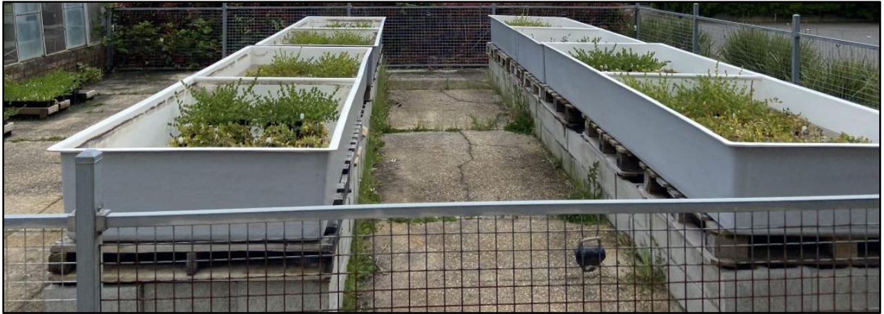
Figure 2 Four waterlogging tanks used to apply treatments. Each tank is separated in two with a waterlogged and control treatment bay.
