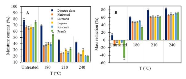
Figure 5. Effect of biomass type and treatment temperature on moisture (A) and mass reduction (B) of digestate. Reaction conditions: digestate/biomass total solid ratio, 1:1; treatment temperature, 180 °C; treatment time, 1 h
