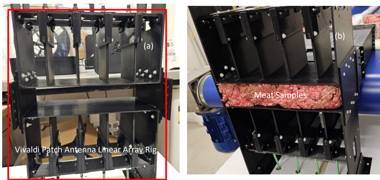
Figure 3: (a) The Vivaldi Patch Antenna Linear Array Rig mounted on food grade materials. (b) The Rig on testing platform on conveyor system with meat samples.
