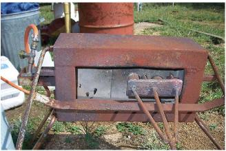
An example of a gas-fired branding furnace.
