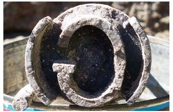
A symbol brand: the face of this one should be filed flat before being used.
