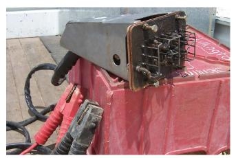
A battery-powered electric branding iron.
