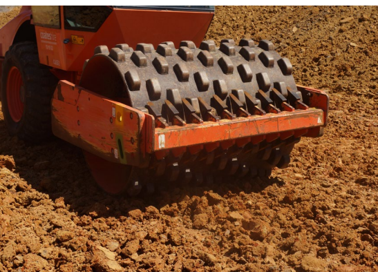
Clay liners should be compacted with at least eight passes of a sheepsfoot roller.
