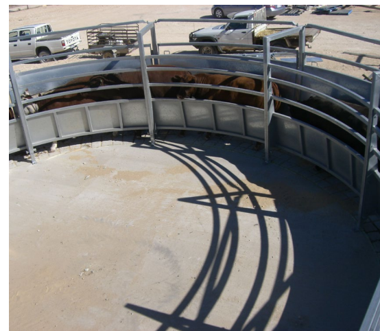
Sheeting on the sides of a race eliminates baulking from visual distractions.
