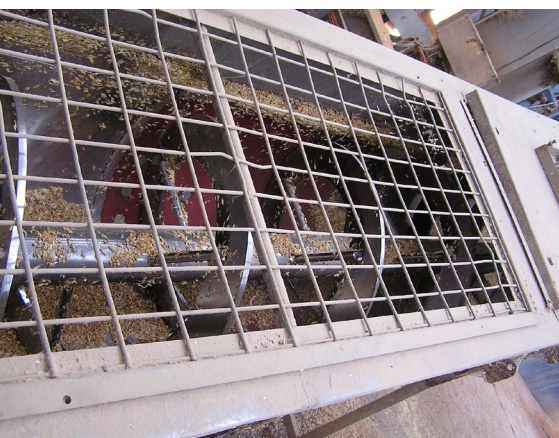
An open spiral mixing auger to convey and mix the grain from the storage silo past the grain-wetting station to the tempering silos.
