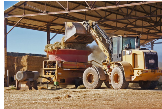
Electric powered semi-permanent tub grinder.
