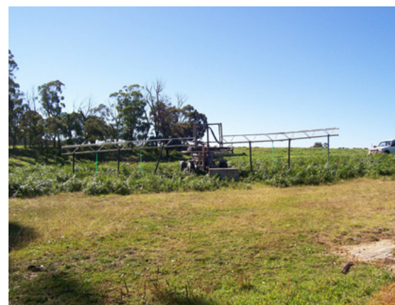
Travelling drip irrigators can apply effluent evenly at low rates.
