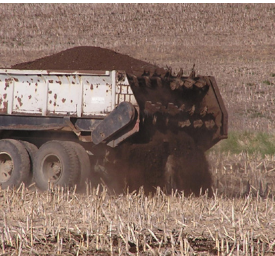
A horizontal beater manure spreader
