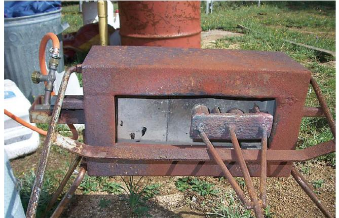
An example of a gas-fired branding furnace.
