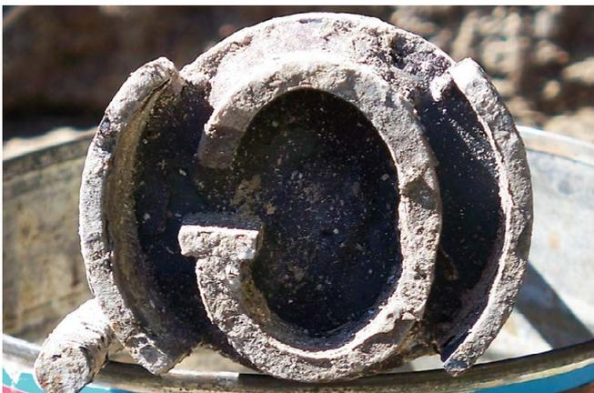
A symbol brand: the face of this one should be filed flat before being used.
