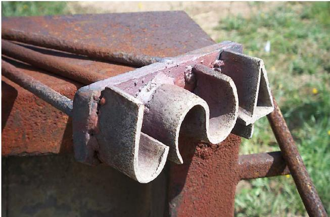
A conjoined three-piece brand is quicker to use than three separate brands and causes less distress.
