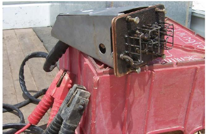
A battery-powered electric branding iron.
