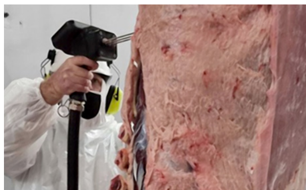
▲ Hot grading measurement provides individual carcass marble scores within two hours of slaughter, supporting same-day chiller sorting, boning runs and market allocation while reducing energy and chiller space costs.
